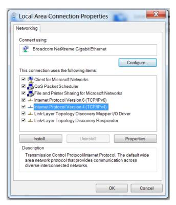
Then near the top, click on "Use the following IP address" - set the IP address to read 10.0.0.X, where X is any number between 0 and 255. The Subnet Mask should then automatically change to 255.0.0.0; if not, simply type this in and then click Ok.
