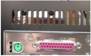
Switch on the console and check that the fan runs free Close the console and tighten the Dzus screws.
