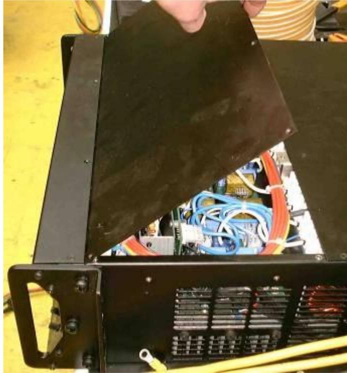
Check that both strips have “stuck” to the cover before finally fixing the cover to the dimmer.
