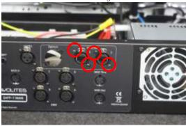
5. Remove the M3 nut holding the earth wires in place, next to the DMX boards. This may be easier if the nearby RJ45 and DVI cables are temporarily removed.
