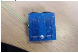
8. Run the earth wire behind the two hex pillars, put the crimp over the earth stud and refit the M3 nut, ensuring all four earth wires are in place, and in contact with one another. (Note that consoles fitted with a DC-UPS will have a fifth earth wire on the stud, which also needs refitting).
